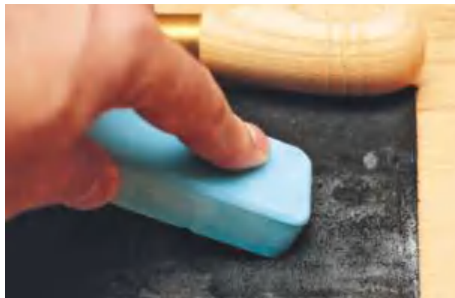
▲ The honing compound is quite hard and chalky when applying to the leather
